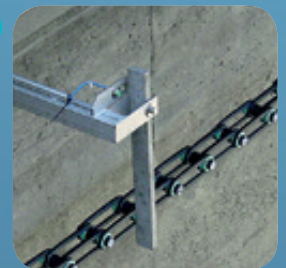
Flight alignment monitoring system
