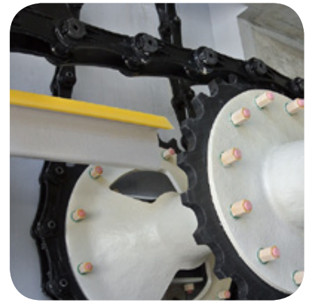
Shaft and flange made from GRP
